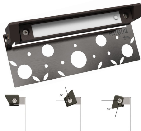
The pivoting head can be angled down to 75° and up to 70°
